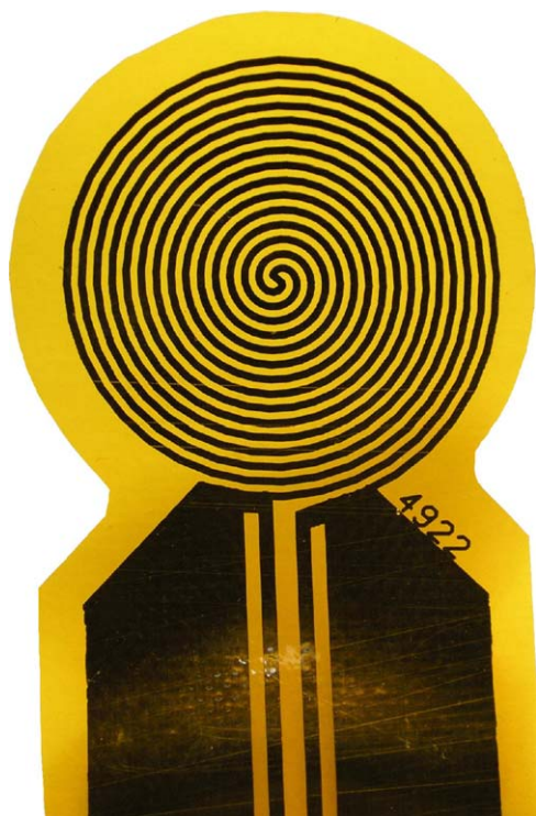
Fig. 3. Hot Disk sensor. The sensor insulation is Kapton of 25 \mu\text{m} thickness on each side. The sensing and heating pattern is made of 12 \mu\text{m} thick Ni.
